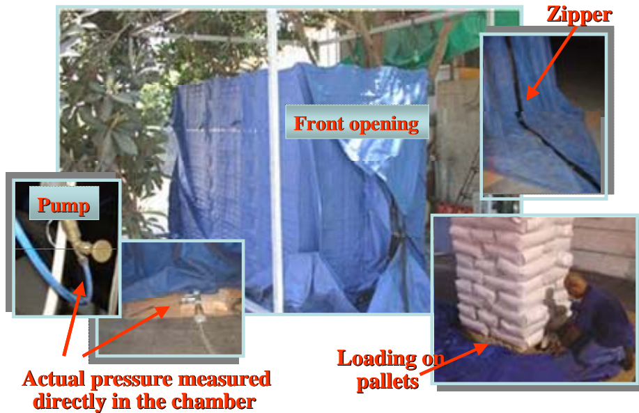
Fig. 2. The V-HF (Vacuum-Hermetic Fumigation) system.
